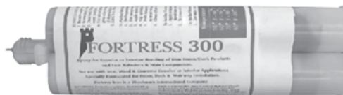
F300 Slow Cure Epoxy 20-30 minute work time. 11 oz. cartridge, will install 60-80 balusters, both ends. Mixing nozzle not included - order F120.
