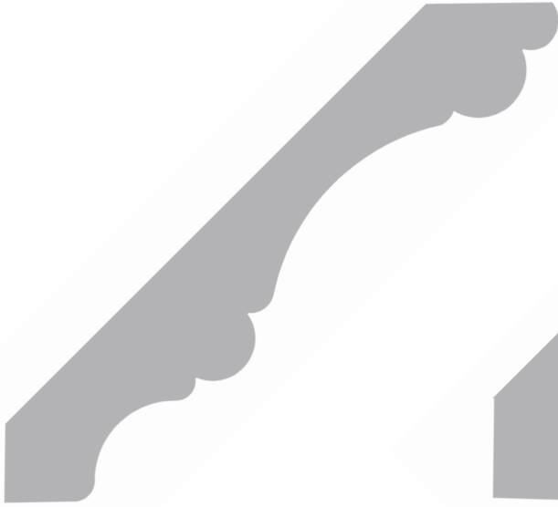
HL342510 \frac{3}{4} " x 4\frac{1}{4} " POPLAR AND FJ POPLAR Rise: 2\text{-}13/16 " Run: 3\text{-}3/16 "
