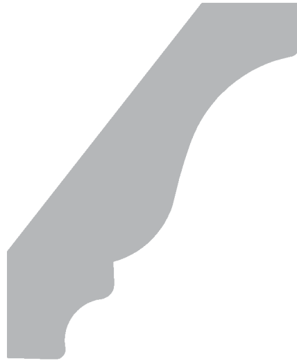
HL3325 \frac{3}{4} " x 3\frac{1}{4} " RED OAK AND POPLAR Rise: 2\frac{9}{16} " Run: 2\frac{1}{16} "
